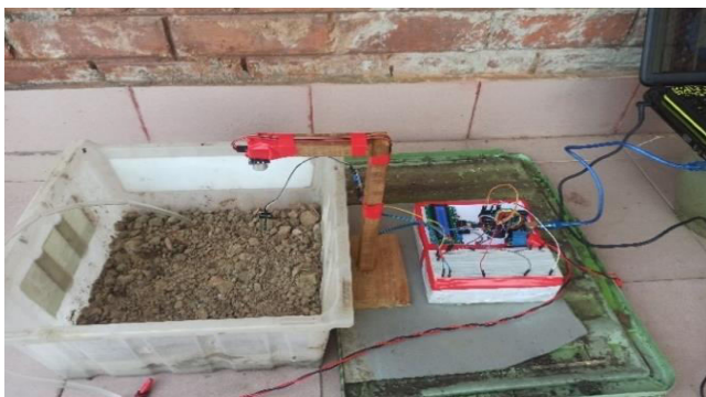
Fig 7: Prototype model for smart irrigation system.
